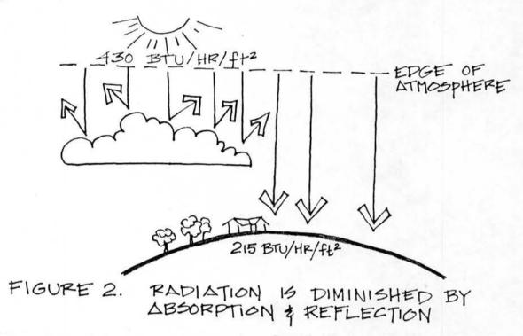
Of the radiation that is reflected some may still reach the earth as diffuse radiation. The amount of radiation absorbed and reflected varies with the composition of the air (water vapor, dust, smog, etc.), and also with the position of the sun. As the length of the sun's path through the atmosphere increases, the amount of reflection and absorption also increase, fig. 3.
