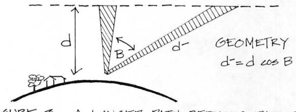
FIGURE 3. A LONGER PATH REDUCES RADIATION RECEIVED
