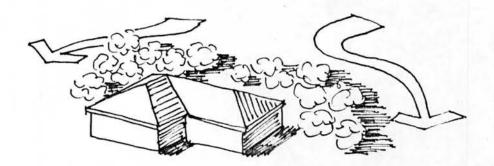
FIGURE 36. VEGETATION PROPERLY PLACED CAN DEFLECT RATHER THAN DAM COLD AIR FLOW
