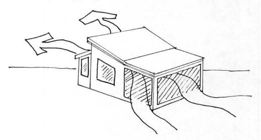
FIGURE 15. SCREENED PORCHES INCREASE VENTILATION
