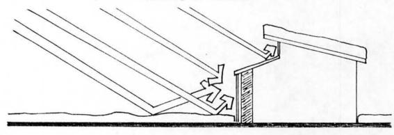
FIGURE 9. SNOW CAN POUBLE RADIATION
