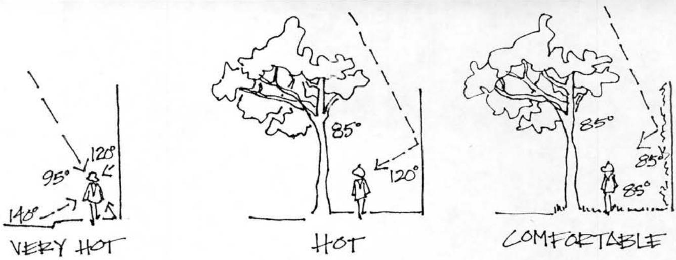
FIGURE 7. SOL-AIR TEMPERATURE - 90° BASE TEMPERATURE
