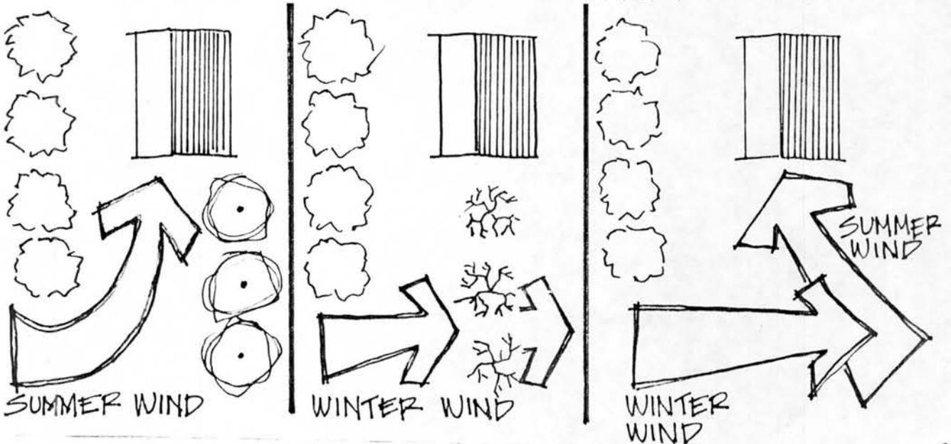
The loss of heat and comfort through conduction and infiltration caused by cold winter winds can be reduced by careful design. Reductions in energy use for heating of up to 30% have been reported from the use of wind breaks, fig.35.
