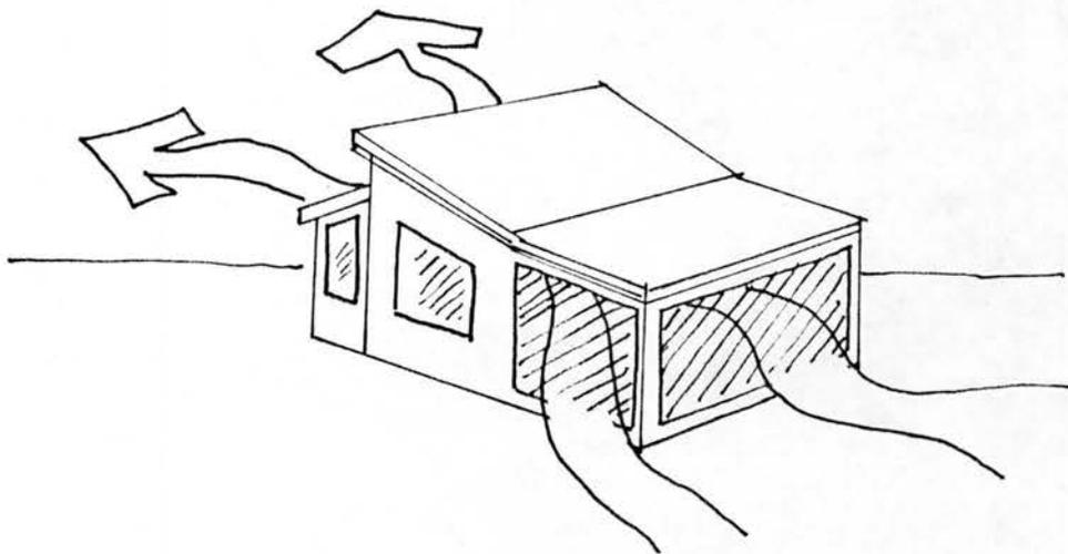
FIGURE 15. SCREENED PORCHES INCREASE VENTILATION
