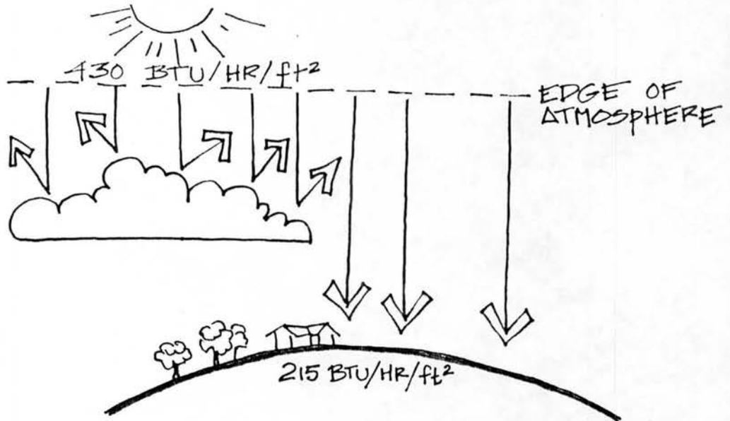
FIGURE 2. RADIATION IS DIMINISHED BY ABSORPTION & REFLECTION
