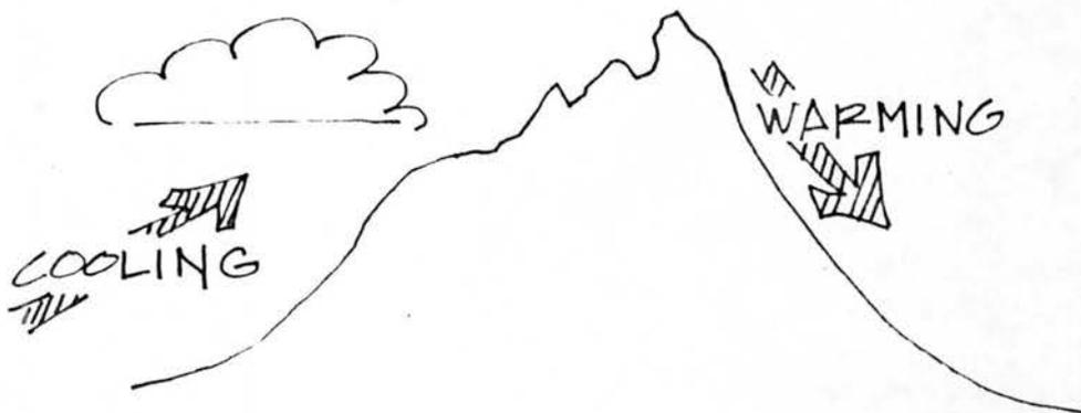
FIGURE 26. AIR MASSES CHANGE TEMPERATURE WITH ALTITUDE
