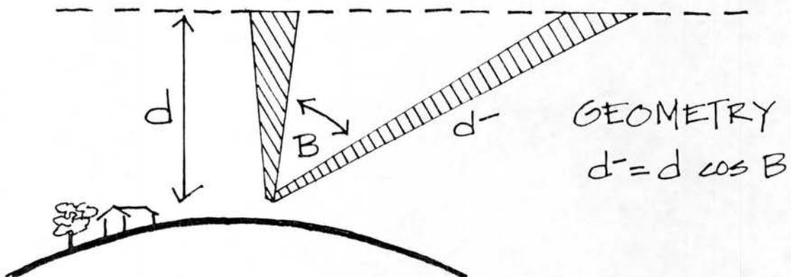
FIGURE 3. A LONGER PATH REDUCES RADIATION RECEIVED
