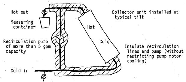
1. Collector should be set up for test as in the diagram:
