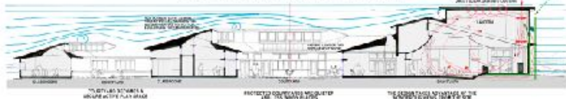
CONFIGURATION FOR NATURAL LIGHTING / VENTILATION & PROTECTION FROM WIND / HIGHWAY NOISE - WEST-SOUTH SECTION 01' = 1'
