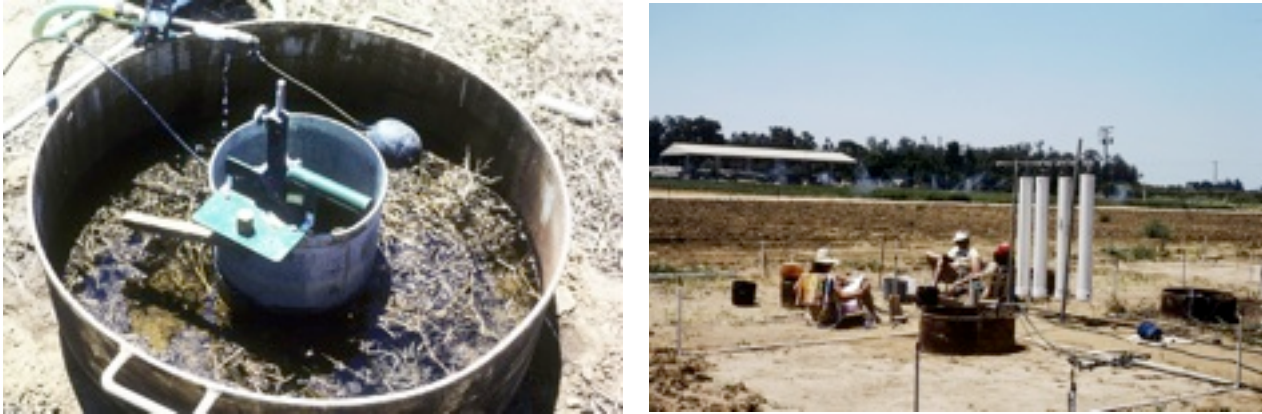
Figure 2. Large double ring infiltrometer tests
